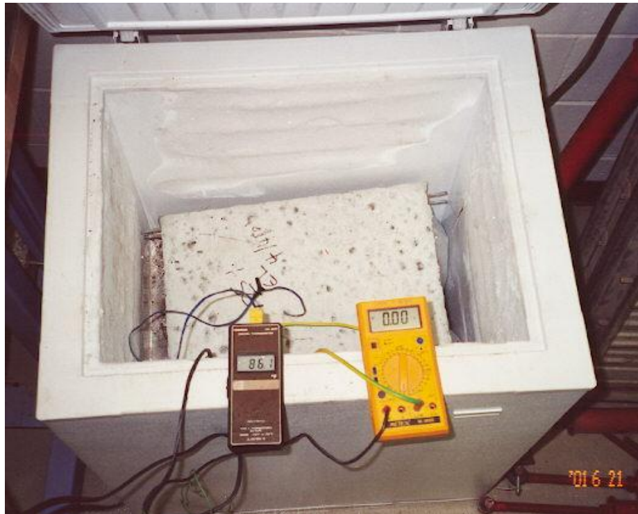
Figure 2. Heating tests conducted with slabs in the freezer
